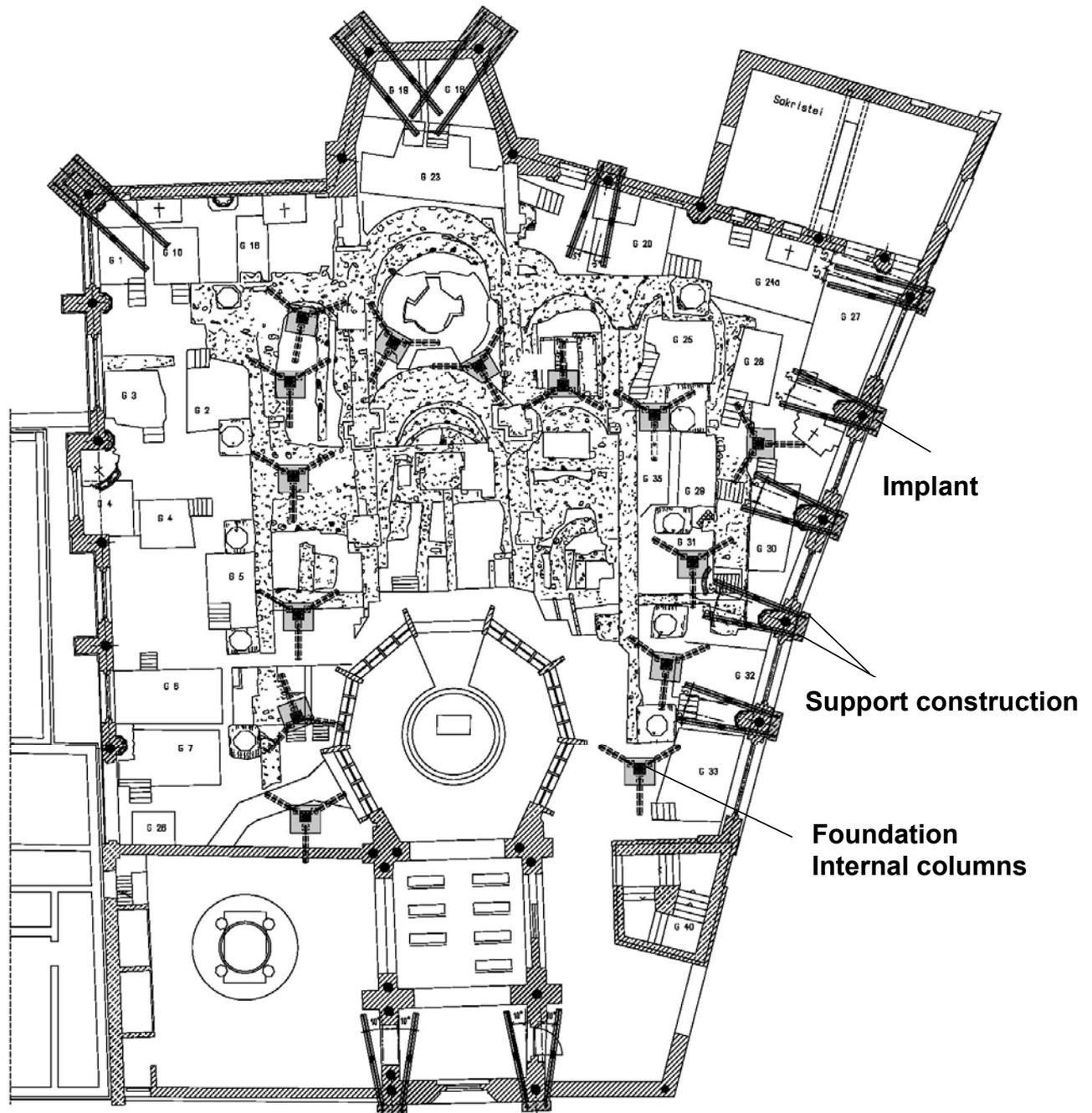
**Fig. 11:** Plan view with foundations in digging field and external wall implants
